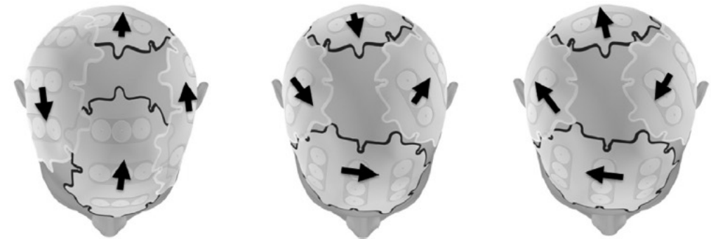
Figure 8. Preventive measures. Illustration of shifting transducer arrays at each array exchange.
